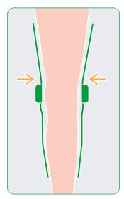
When adjusting the hinge rods to the shape of the extremity by using an orthopaedic bending iron, you must not bend the rods in the area of the hinge housing or the hinge cover as this could lead to damage or break of the hinge.
